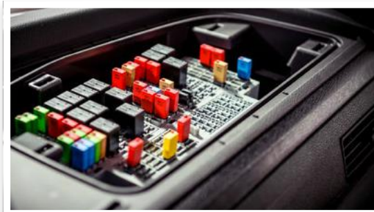
In-cab electrical panel
